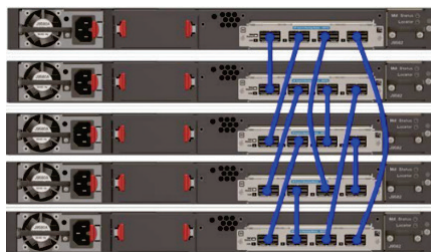
Figure 6. HP 3800 Switch Series physical stacking
